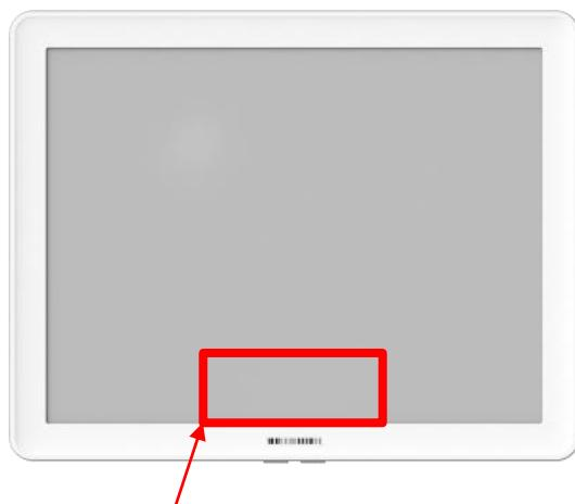
**A remote controller or a NFC Device contact point for communication.**
