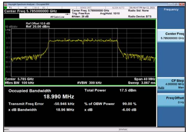
U-NII-3 6dB Bandwidth-802.11ax(20MHz) ,5825MHz,Ant1
