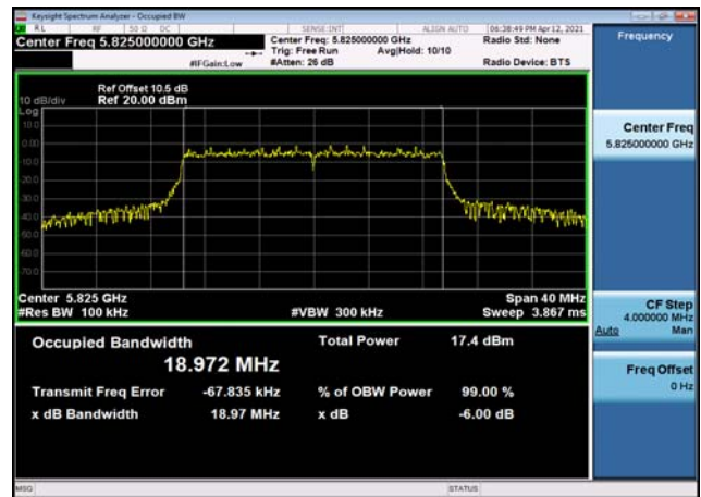
U-NII-3 6dB Bandwidth-802.11ax(40MHz) ,5755MHz,Ant1
