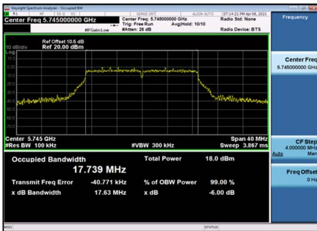
U-NII-3 6dB Bandwidth-802.11ac(20MHz) ,5745MHz,Ant1
