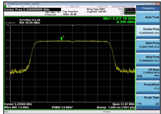
U-NII-1 Power spectral density-802.11 ax(20MHz),5240MHz,Ant1
