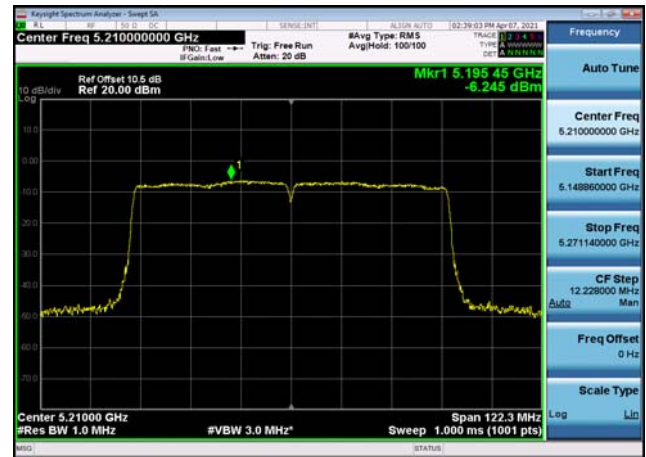
U-NII-1 Power spectral density-802.11 ax(20MHz),5180MHz,Ant1
