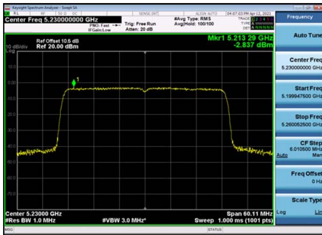
U-NII-1 Power spectral density-802.11 ax(80MHz),5210MHz,Ant0
