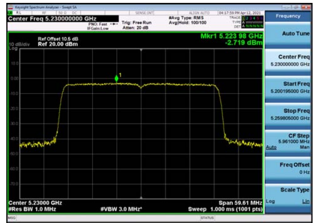
U-NII-1 Power spectral density-802.11 ax(80MHz),5210MHz,Ant1
