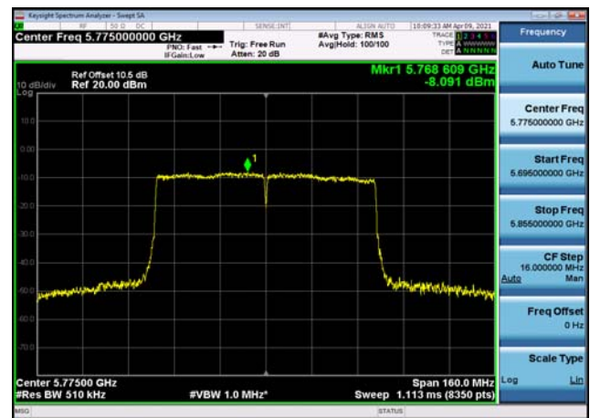
U-NII-3 Power spectral density-802.11 ac(80MHz),5775MHz,Ant0
