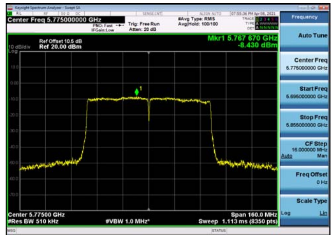
U-NII-3 Power spectral density-802.11 ax(20MHz),5745MHz,Ant1
