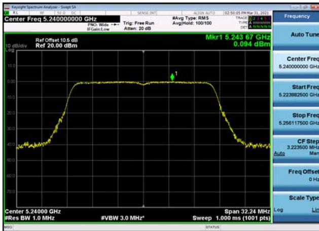
U-NII-1 Power spectral density-802.11 ac(40MHz),5230MHz,Ant1
