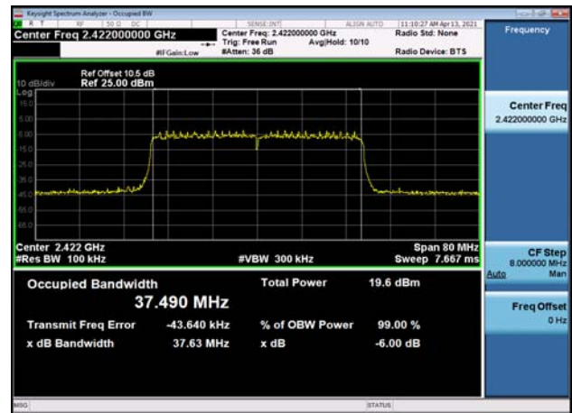
6dB Bandwidth-802.11ax(HE40),2437MHz ,Ant1
