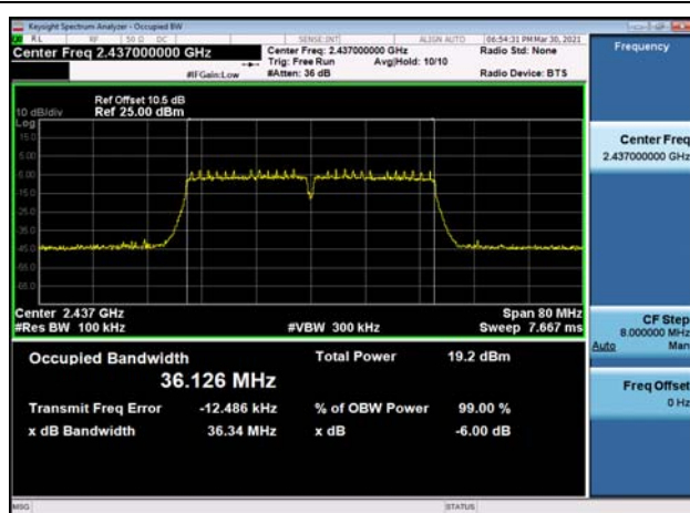
6dB Bandwidth-802.11n(HT40),2437MHz
