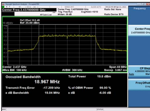
6dB Bandwidth-802.11ax(HE20),2462MHz ,Ant0
