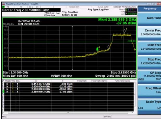
,Plot 2,Band Edge-802.11g,2462MHz ,Ant0
