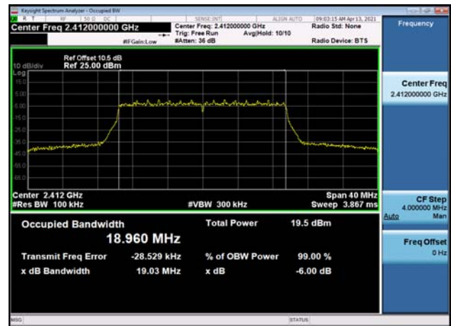
6dB Bandwidth-802.11ax(HE20),2437MHz ,Ant1
