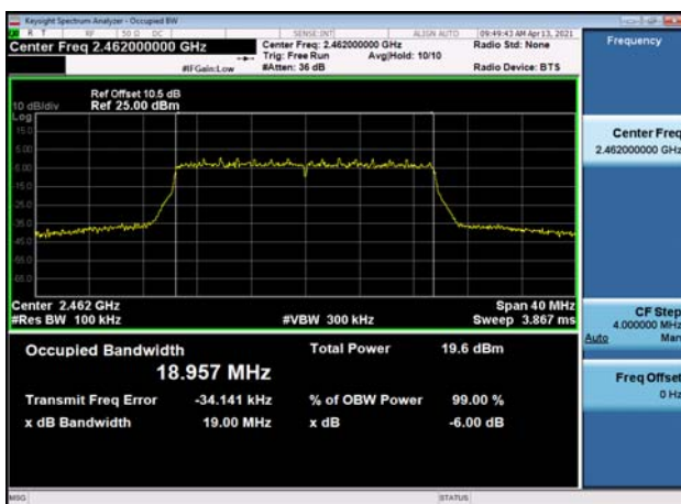
6dB Bandwidth-802.11ax(HE20),2462MHz ,Ant0
