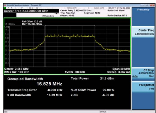
6dB Bandwidth-802.11g,2462MHz,Ant1
