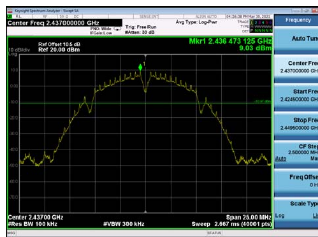
,Plot 2,Band Edge-802.11b,2412MHz ,Ant0
