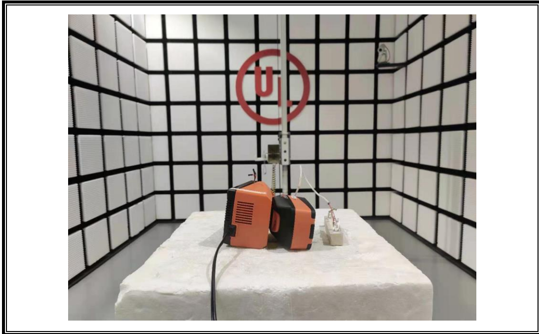
POWERLINE CONDUCTED EMISSIONS MEASUREMENT SETUP
