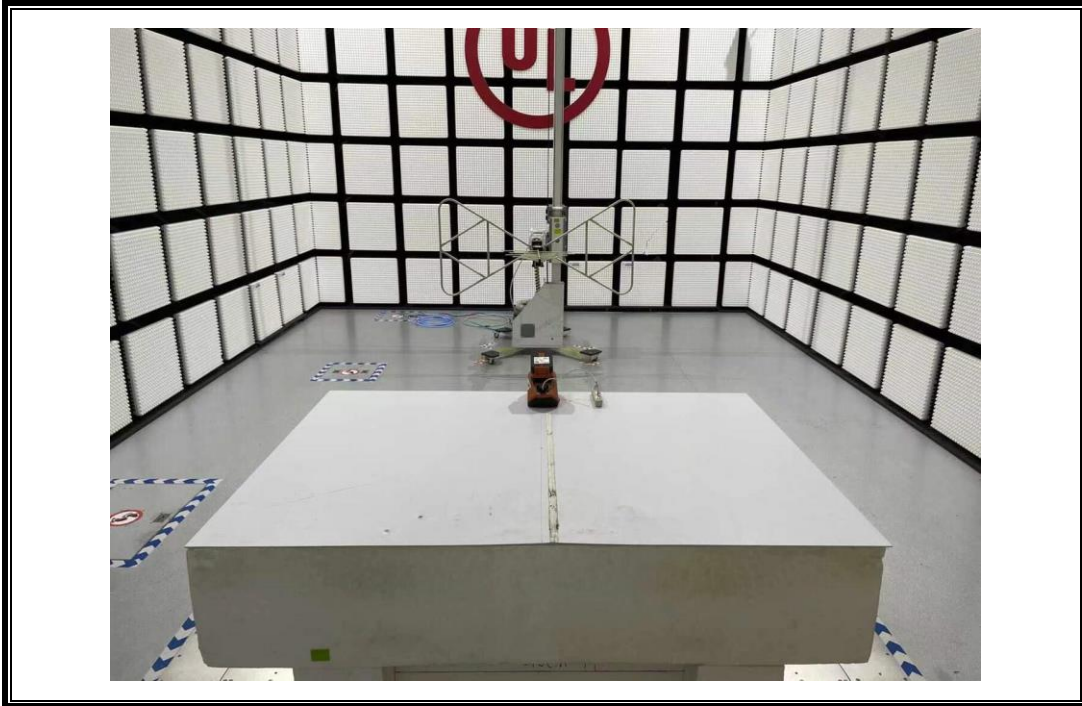
RADIATED RF MEASUREMENT SETUP (30MHz ~ 1 GHz)
