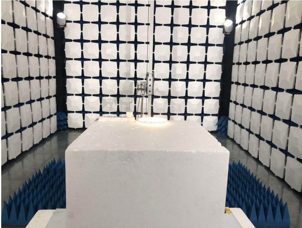
Above 1GHz for radiated emission test setup
