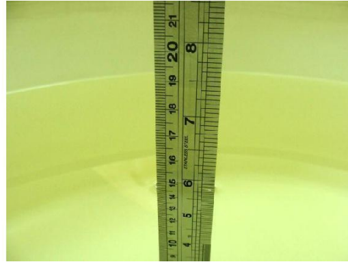
Fig 7.2 Photo of Liquid Height for Body SAR
