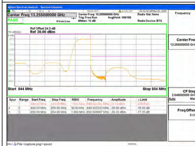
B26 Part22 / 5MHz / High CH / QPSK / 1 RB
