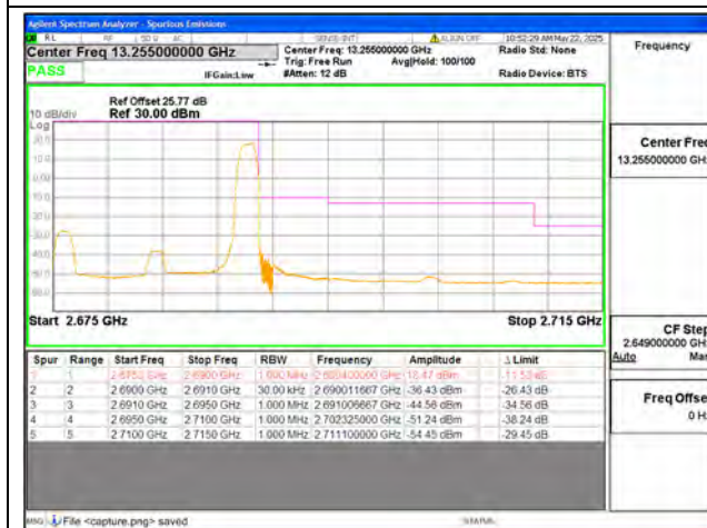
B41 / 15MHz / High CH / QPSK / 1 RB
