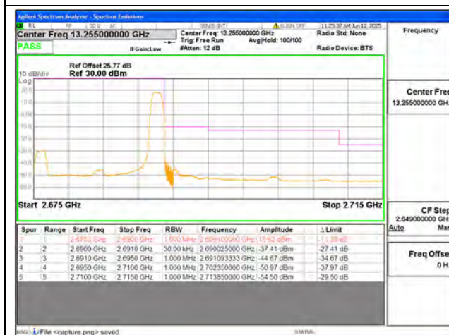
B41 / 15MHz / High CH / QPSK / 1 RB
