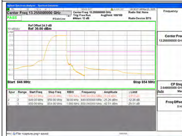
B26 Part22 / 1.4MHz / High CH / QPSK / 1 RB
