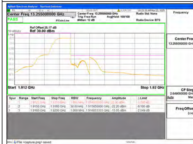
B25 / 1.4MHz / High CH / QPSK / 1 RB
