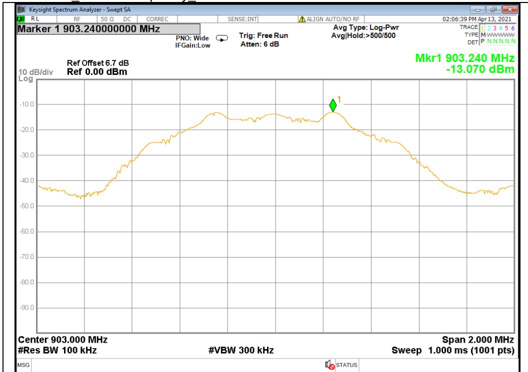
Test mode : GFSK\_Lowest Frequency\_Bandedge
