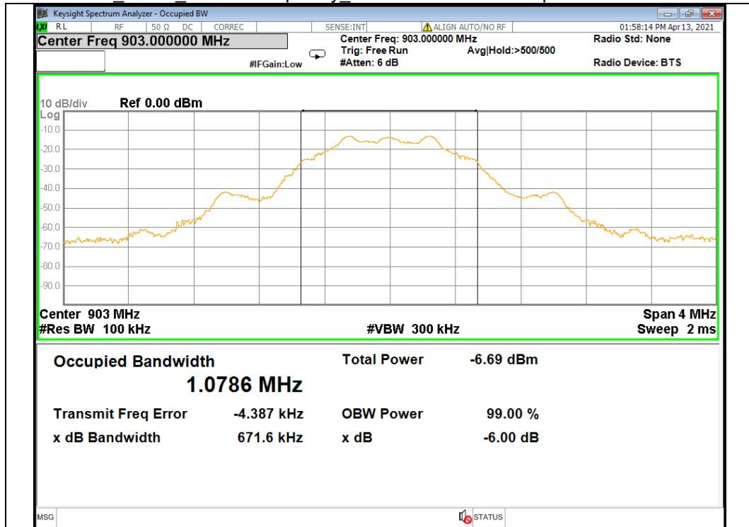
Test mode : GFSK Middle Frequency 6 dB Bandwidth / Occupied Bandwidth
