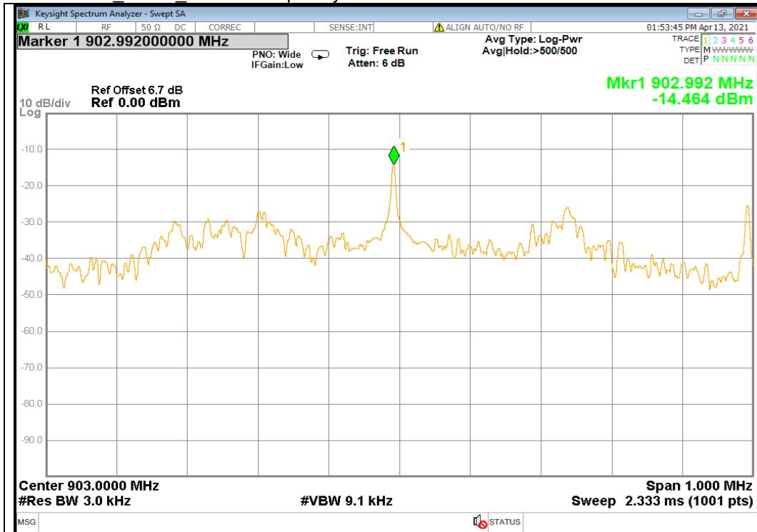
Test mode : GFSK\_Middle Frequency
