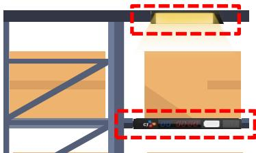
Attach it to each cell to use LED lights that work with the indicator to increase visibility of the operator to prevent job errors.
