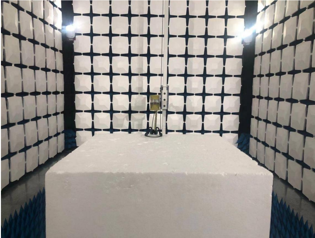
Above 1GHz for radiated emission test setup
