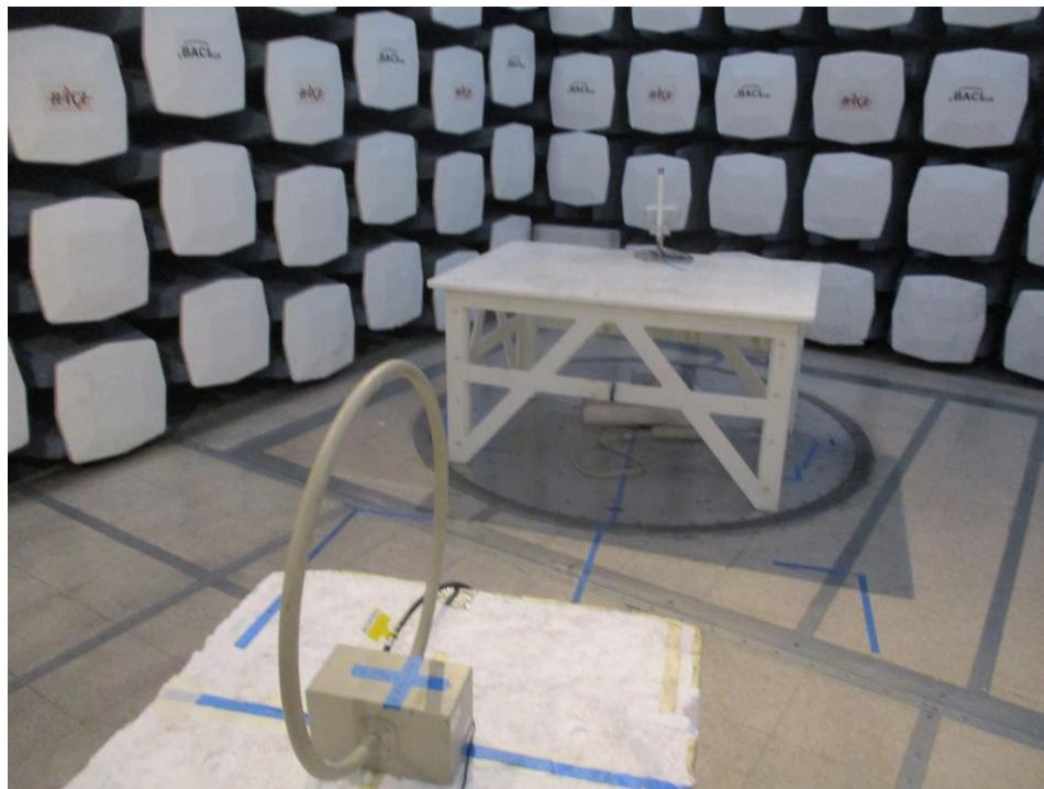
**1.6 Spurious Radiated Emissions: 9 kHz to 30 MHz, Parallel, Rear View at 3 meters distance
