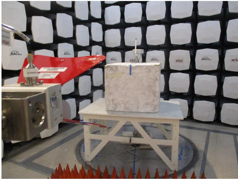
**1.16 Spurious Radiated Emissions: 1 GHz to 18 GHz, Rear View at 3 meter distance (Long Range Antenna)**
