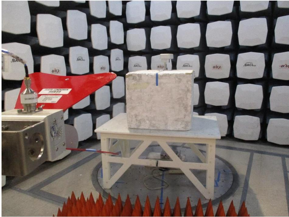
**1.14 Spurious Radiated Emissions: 1 GHz to 18 GHz, Rear View at 3 meter distance (Short Range Antenna)**
