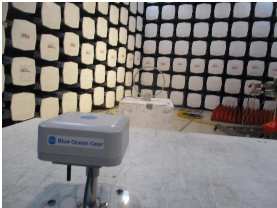
**1.5 Spurious Radiated Emissions: 9 kHz to 30 MHz, Parallel, Front View at 3 meters distance
