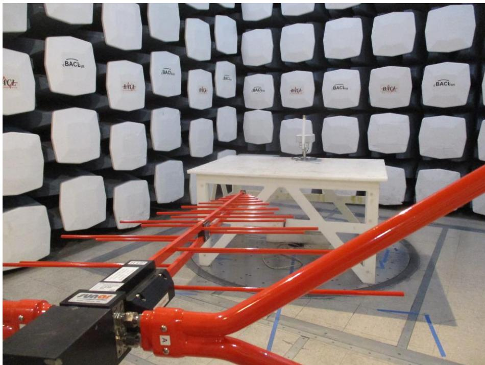
**1.12 Spurious Radiated Emissions: 30 MHz to 1000 MHz, Rear View at 3 meters distance (Long Range Antenna)**
