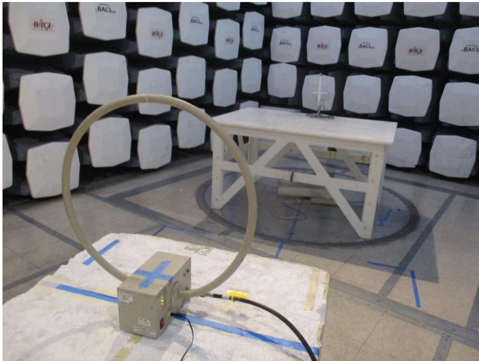
**1.8 Spurious Radiated Emissions: 9 kHz to 30 MHz, Perpendicular, Rear View at 3 meters distance (Long Range Antenna)**
