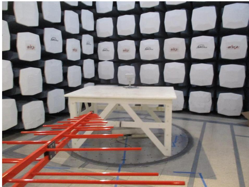
**1.10 Spurious Radiated Emissions: 30 MHz to 1000 MHz, Rear View at 3 meters distance (Short Range Antenna)**
