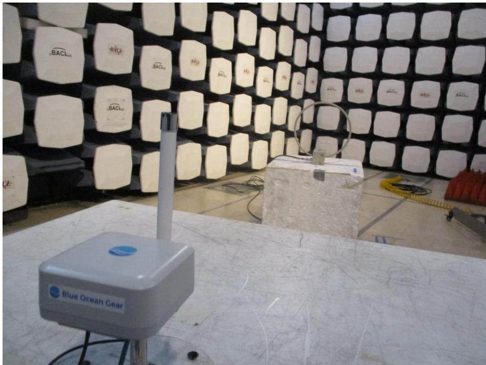
**1.9 Spurious Radiated Emissions: 30 MHz to 1000 MHz, Front View at 3 meters distance
