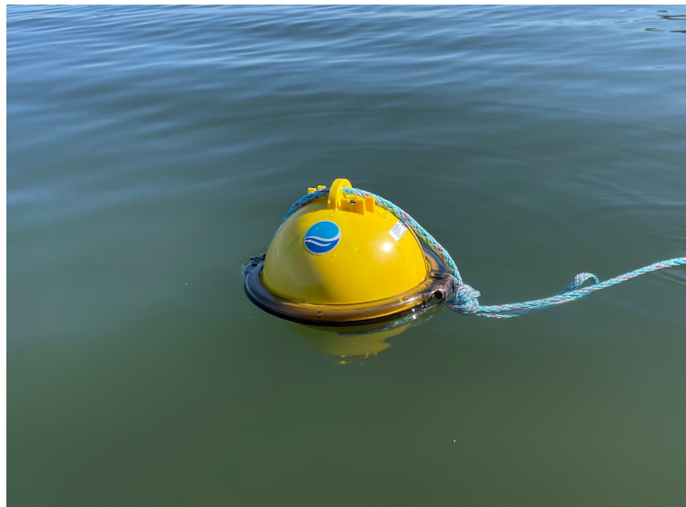
Figure 4: Smart buoy correct orientation while floating.
