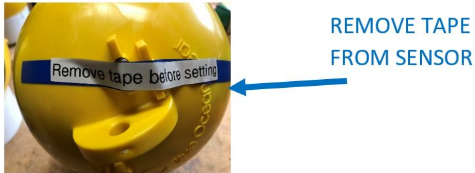
Figure 3: Tape to remove off of sensor before use.
