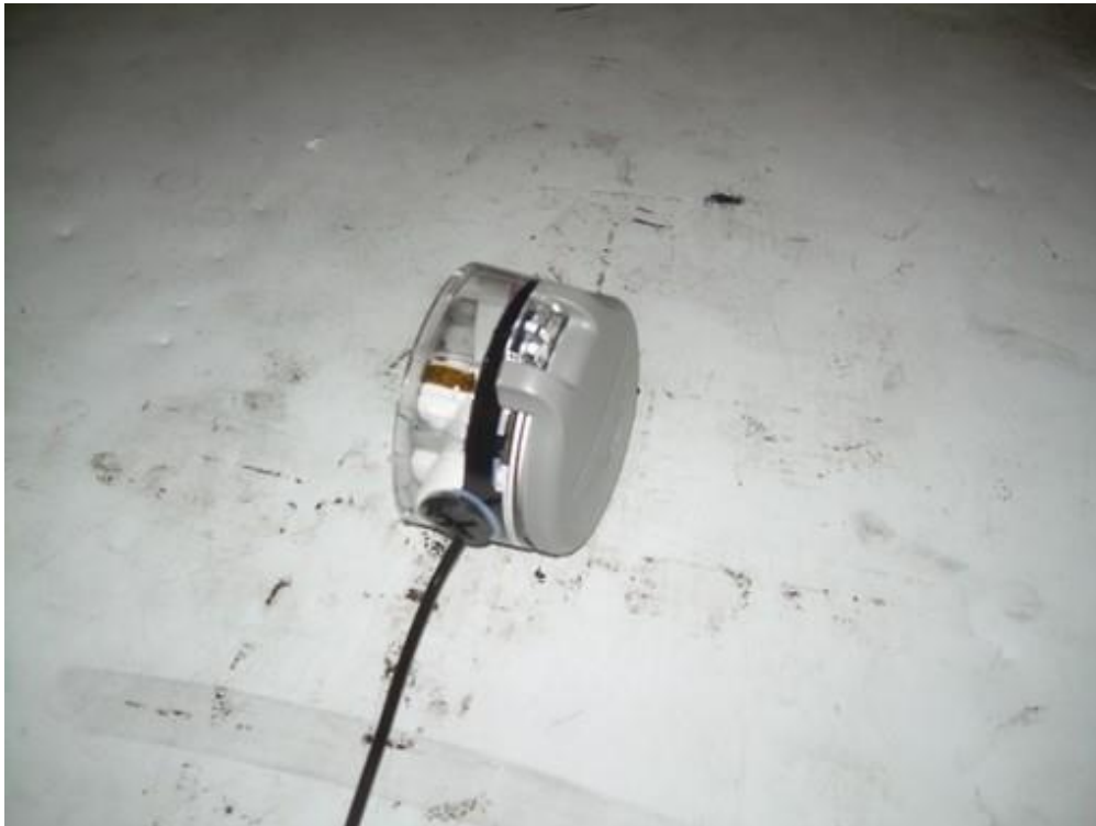
Photograph 6: Radiated Emissions Configuration – Vertical
