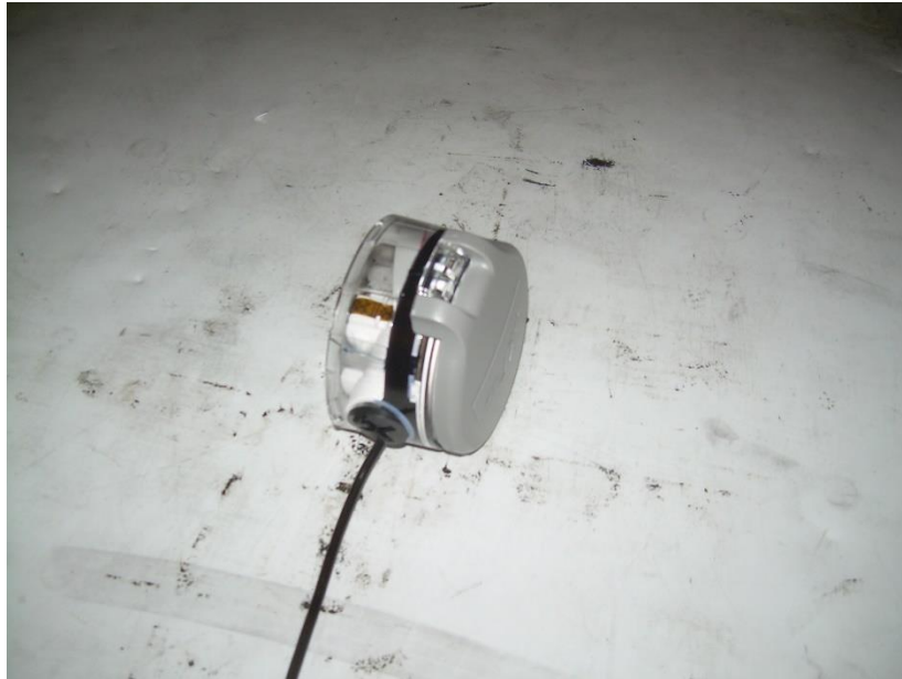
Photograph 3: Radiated Emissions Worst-Case Configuration – Vertical as if Wall Mounted
