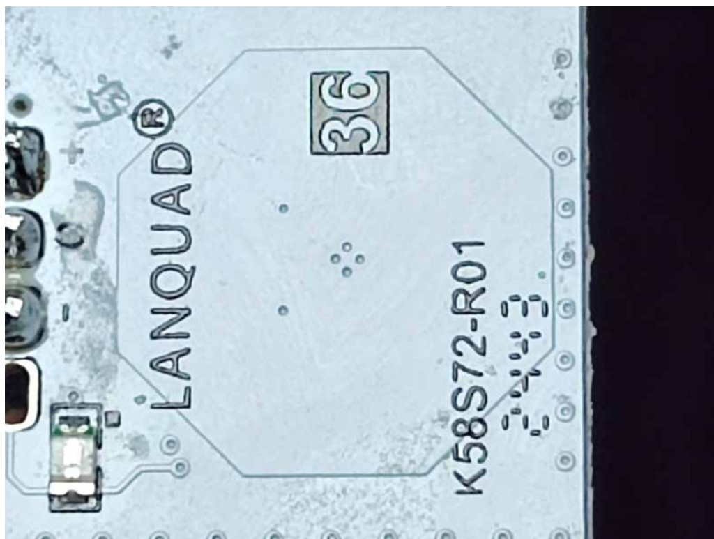
FIGURE 14 LED LAMP (G117P38MO6C) ANTENNA ON CONTROL BOARD
