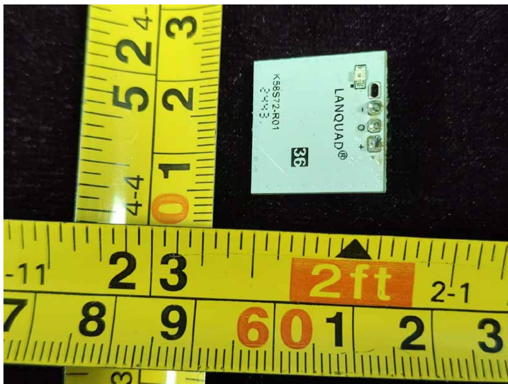
FIGURE 14 LED LAMP (G117P38MO6C) ANTENNA ON CONTROL BOARD
