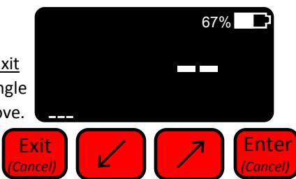
2. Continue to hold down Exit switch until a second bar displays above. Now release switch; unit will power down.
