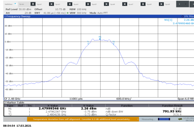
Figure 8.5-3: 6 dB bandwidth on high channel
