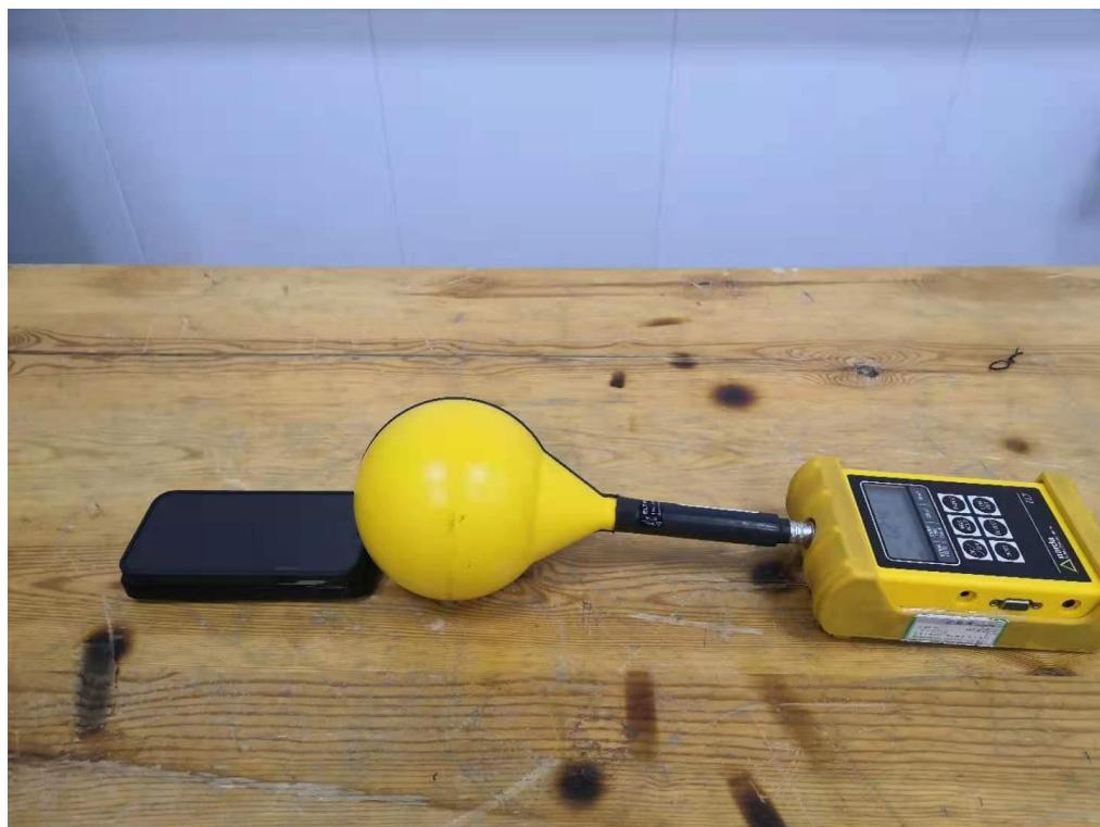
**(TM1)****9.10. Test Position D - Exposure photo from side edge surface-Right (0cm)**
