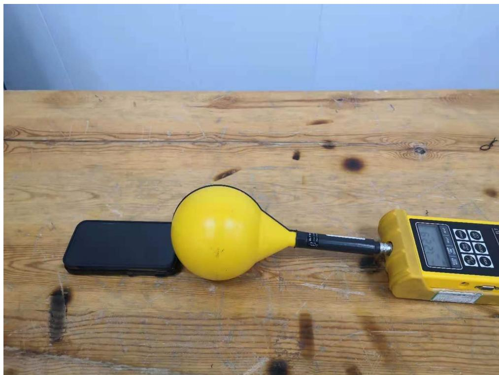
**(TM1)****9.8. Test Position B - Exposure photo from side edge surface-Left (0cm)**
