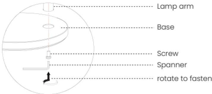
It's very easy to install, as shown above: Insert the lamp arm into the lamp holder and tighten it with hexagon screw from the bottom.
