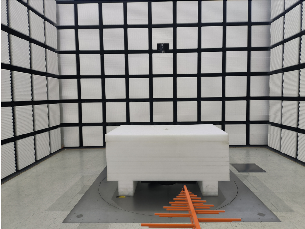
Radiation emission 30MHz to 1GHz recent photograph
