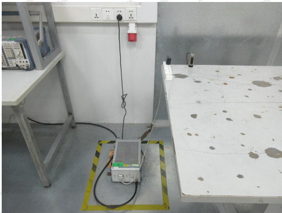
Photo of Power Line Conducted Emission Test
