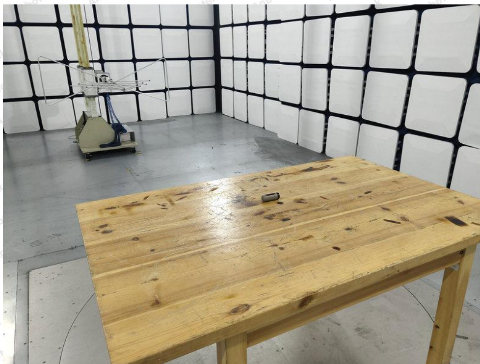
Photo of Radiation Emission Test
