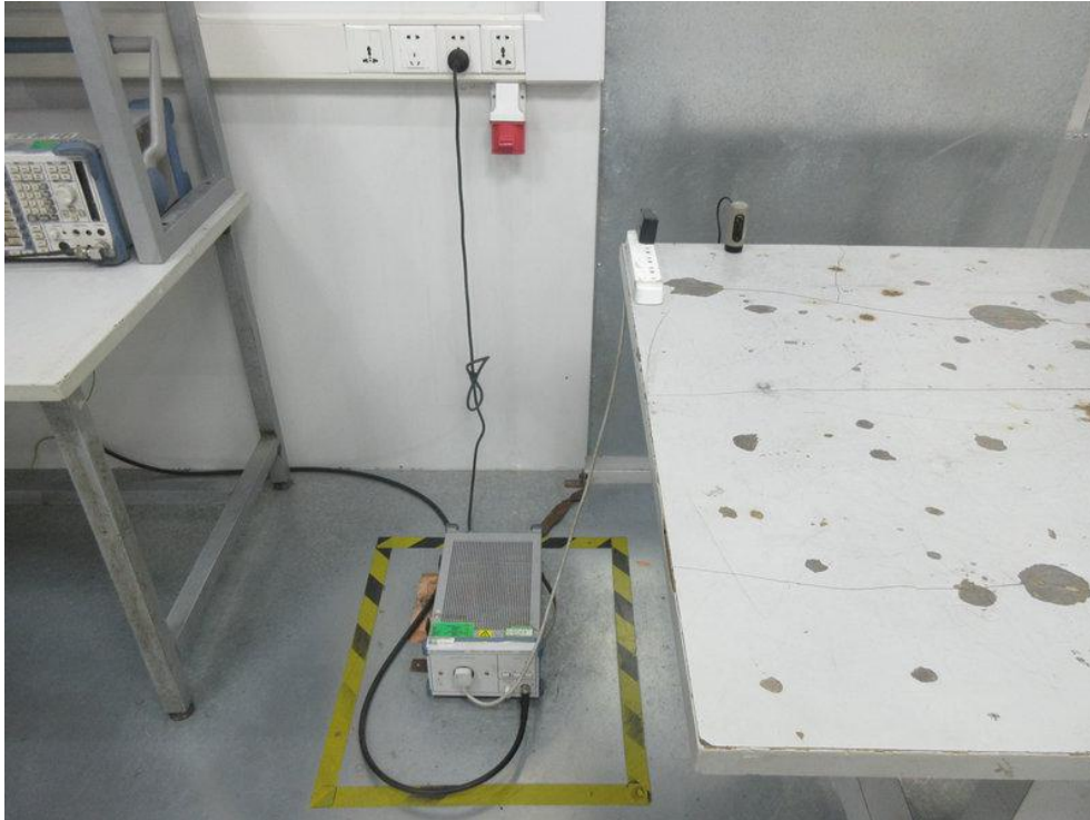
Photo of Power Line Conducted Emission Test
