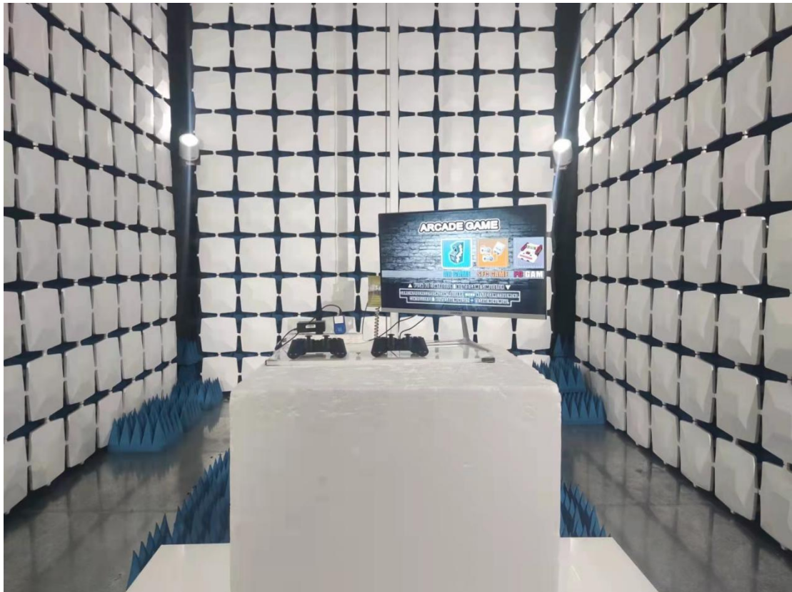
Above 1GHz for radiated emission test setup
