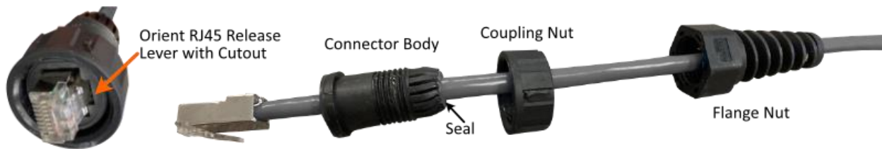
Figure 35: Ethernet Connector Assembly
