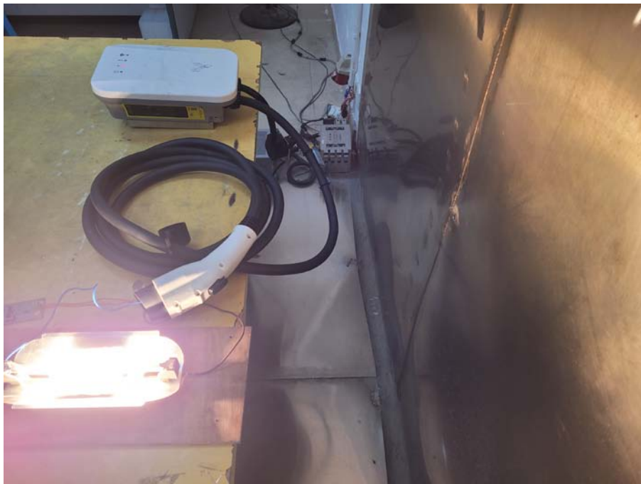
Conducted Emissions Test Setup Side View
