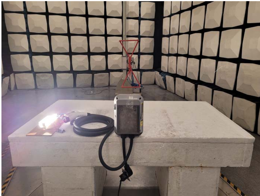
Radiated Emission Rear View (Below 1GHz)
