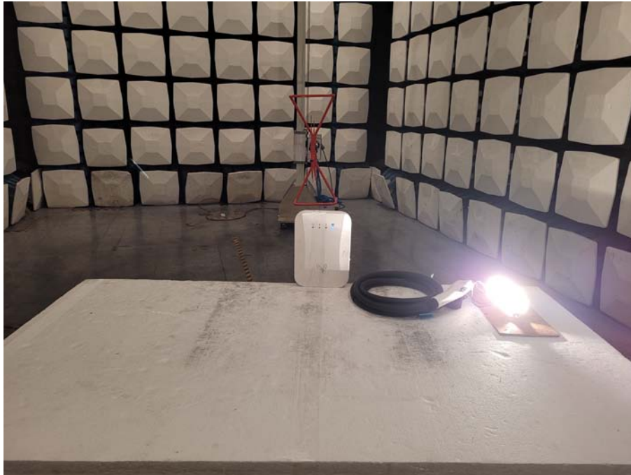
Radiated Emission Front View (Below 1GHz)
