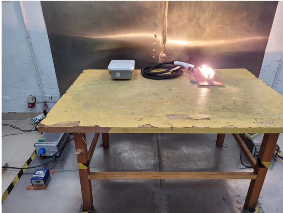
Conducted Emissions Test Setup Front View
