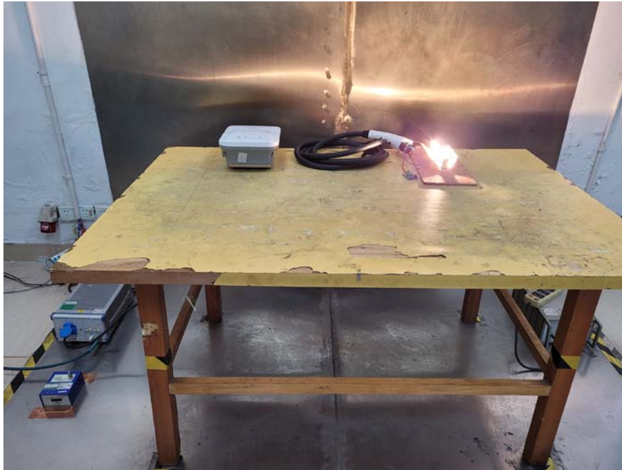
Conducted Emissions Test Setup Front View
