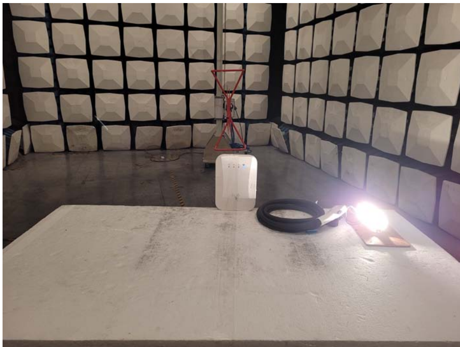
Radiated Emission View (30 MHz-1 GHz)
