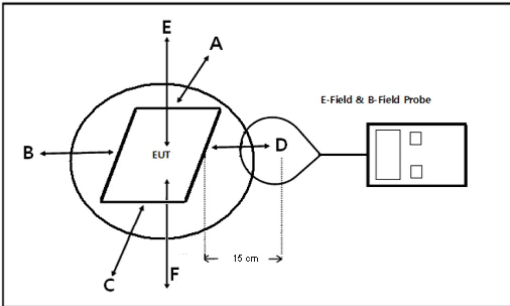
Note: As bottom point is not required to test for desktop devices, so we scanning all the surfaces and recorded the worst level in F.
