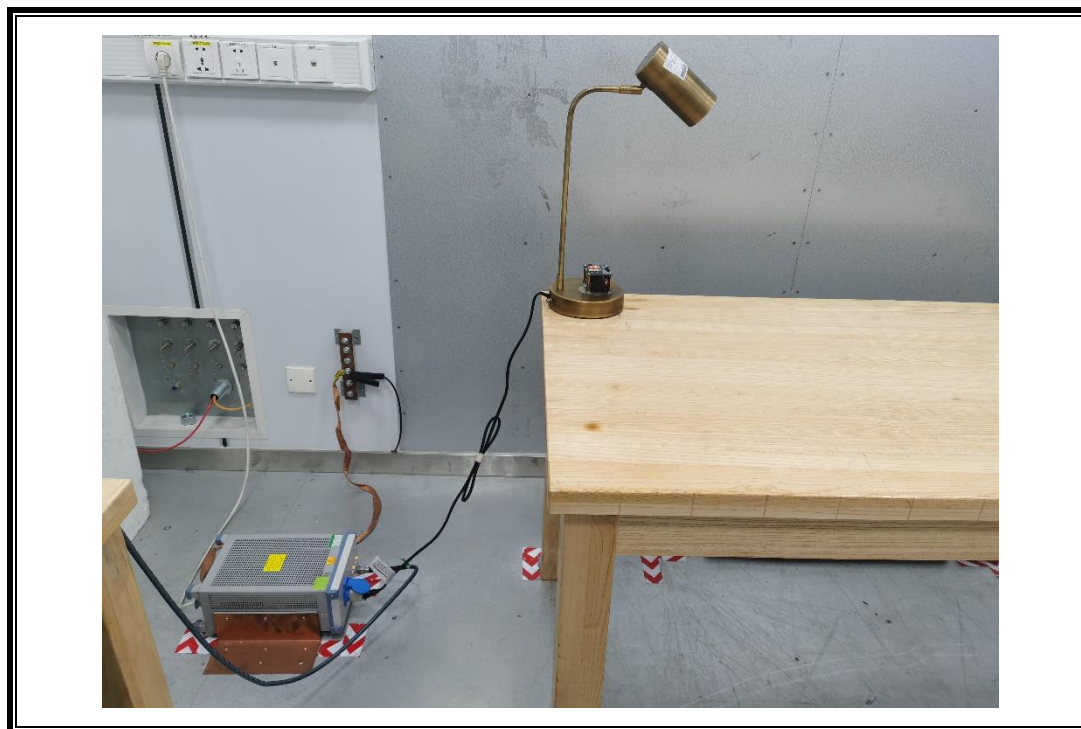
POWERLINE CONDUCTED EMISSIONS MEASUREMENT SETUP
