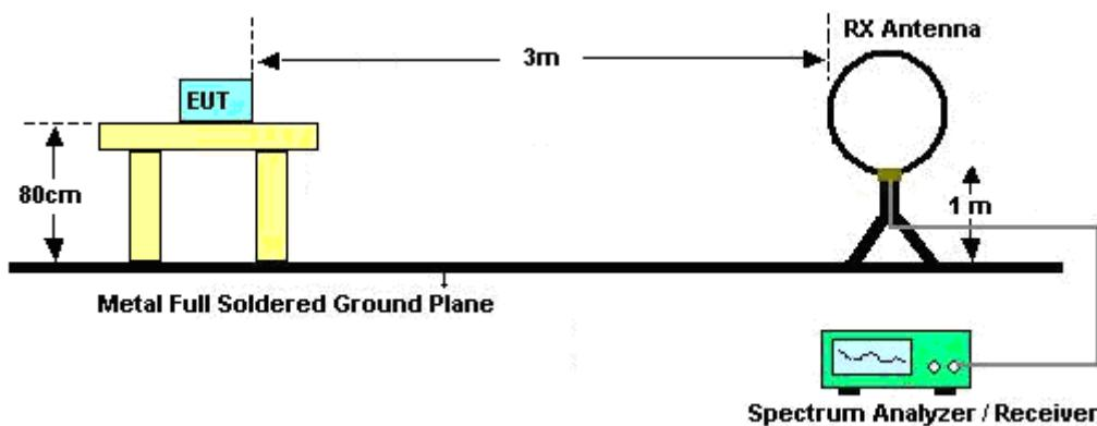
For radiated emissions from 30MHz to 1GHz
