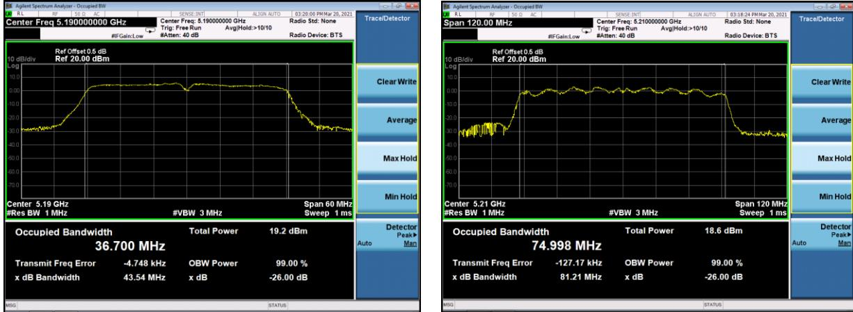
(802.11 AC40) 26dB&99%Bandwidth plot on channel 46
