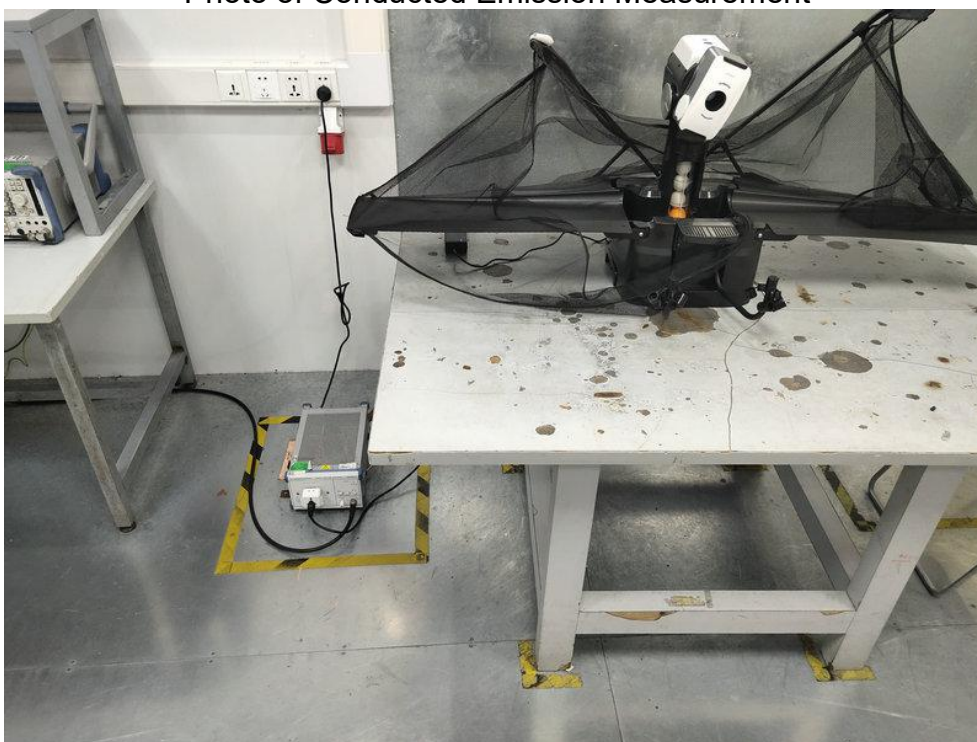
FCC ID: 2AZEZ-ROBOT Photo of Conducted Emission Measurement
