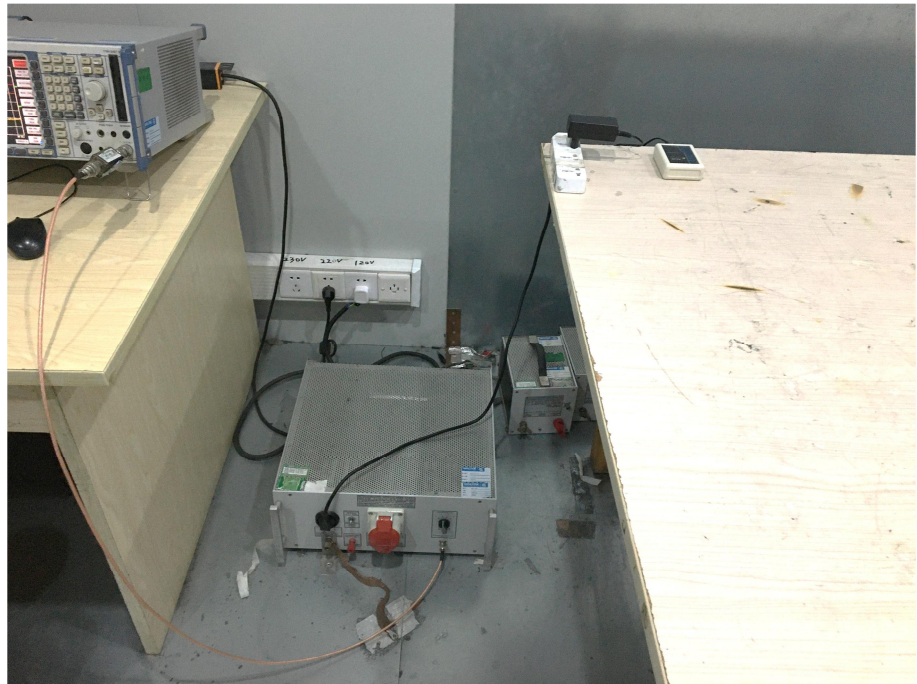
Conducted Emission Test Setup
