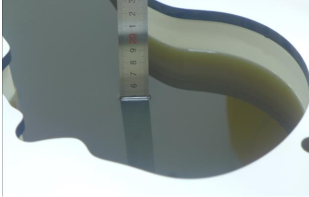
Photo 1: Tissue Simulant Liquid for HBBL600-10000MHz
