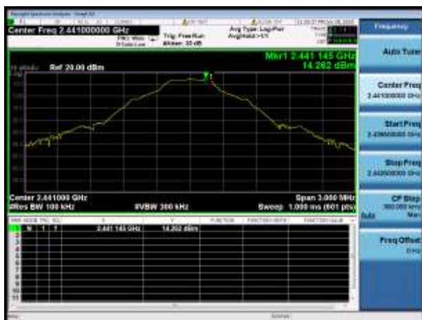
GFSK MIDDLE CHANNEL, CARRIER LEVEL
