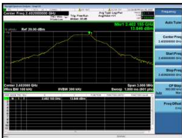
GFSK LOW CHANNEL, CARRIER LEVEL
