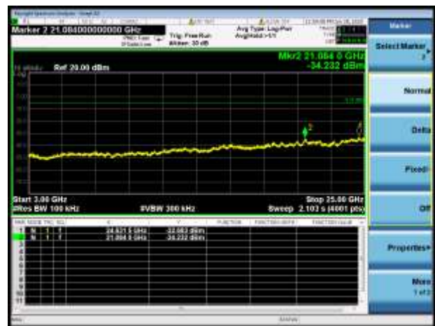
GFSK HIGH CHANNEL, SPURIOUS 3 GHz ~ 25 GHz
