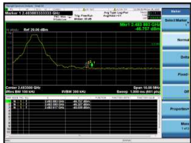
GFSK HIGH CHANNEL, BAND EDGE
