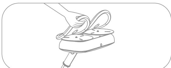
Stick the inner face of mop pads on the wheels at the bottom of the main machine.
