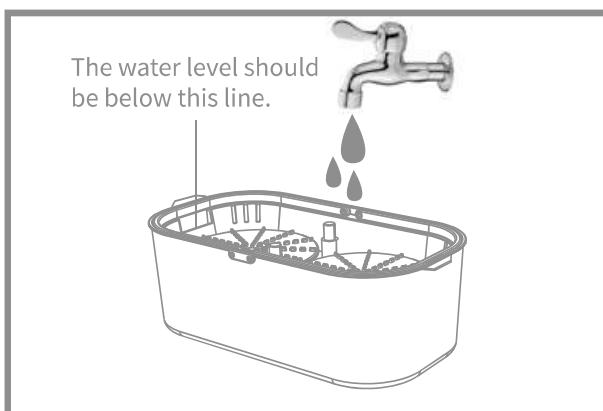
To avoid water overflow into the internal bucket, do not exceed the maximum water level when adding water.
