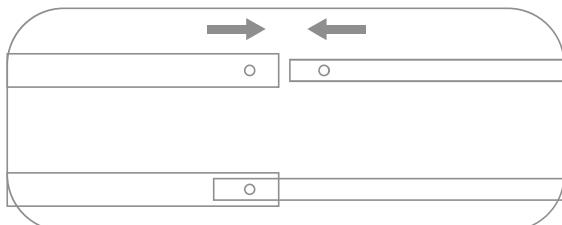
Insert the metal tube into the plastic tube (both ends of the metal tube can be inserted).
