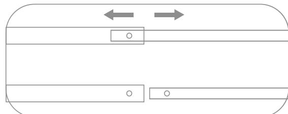
The connected metal and plastic tubes can be disassembled by pressing down the joint point.
