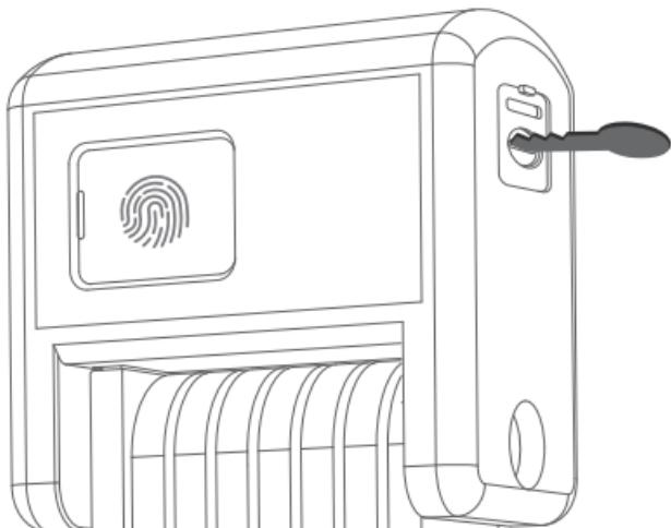
ZiiLock is equipped with two mechanical keys to unlock even if you forget to charge it.
