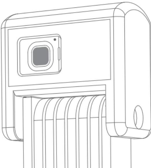
Long press the fingerprint board for about 5 seconds to turn on/off the Bluetooth of ZiiLock. When the lock beeps with a red light, the Bluetooth of the lock is turned off.
