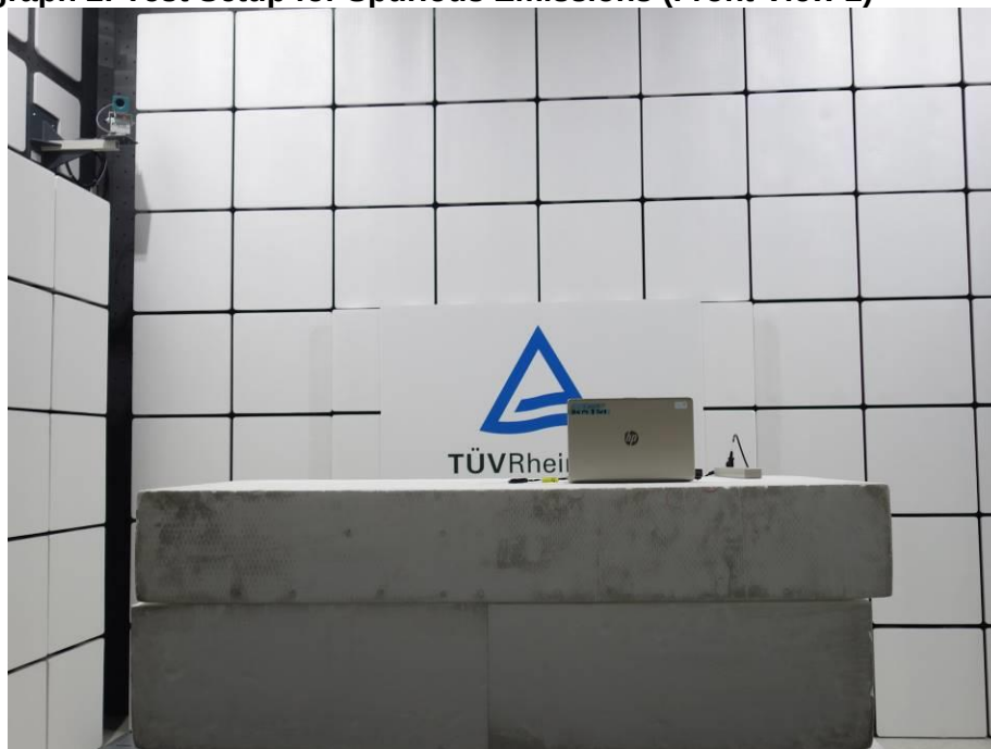
Photograph 2: Test Setup for Spurious Emissions (Front View 2)
