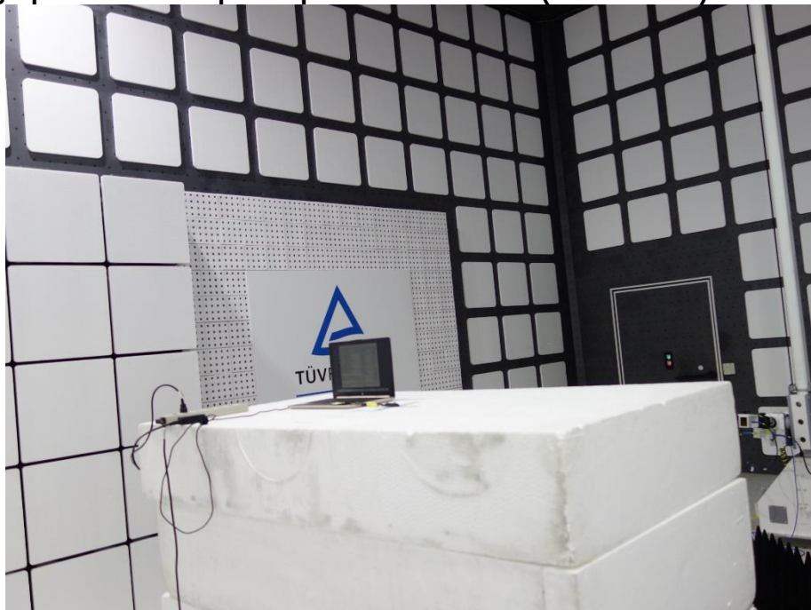
Photograph 6: Test Setup for Spurious Emissions (Back View 4)
