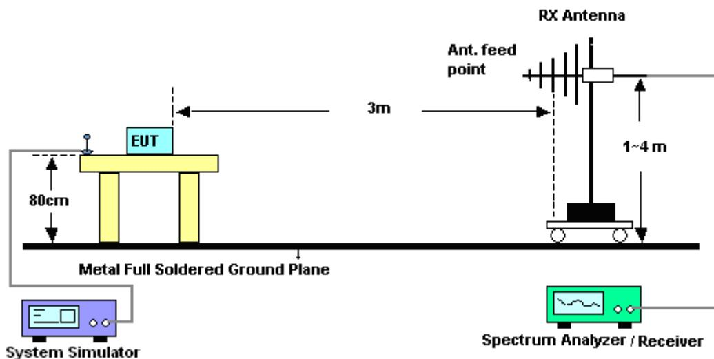
For radiated test above 1GHz
