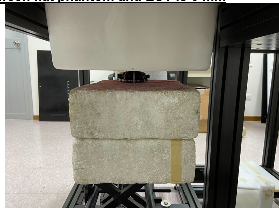
Photograph 4. Product specific 10-g SAR, Front Surface, 0mm
