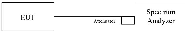
The loss between RF output port of the EUT and the input port of the Spectrum Analyzer has been taken into consideration.
