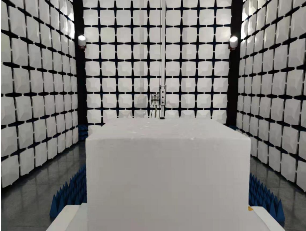
Above 1GHz for radiated emission test setup
