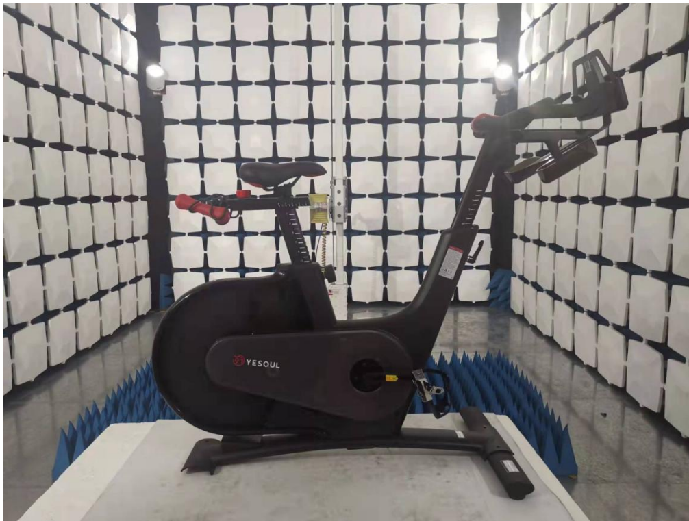
Above 1GHz for radiated emission test setup
