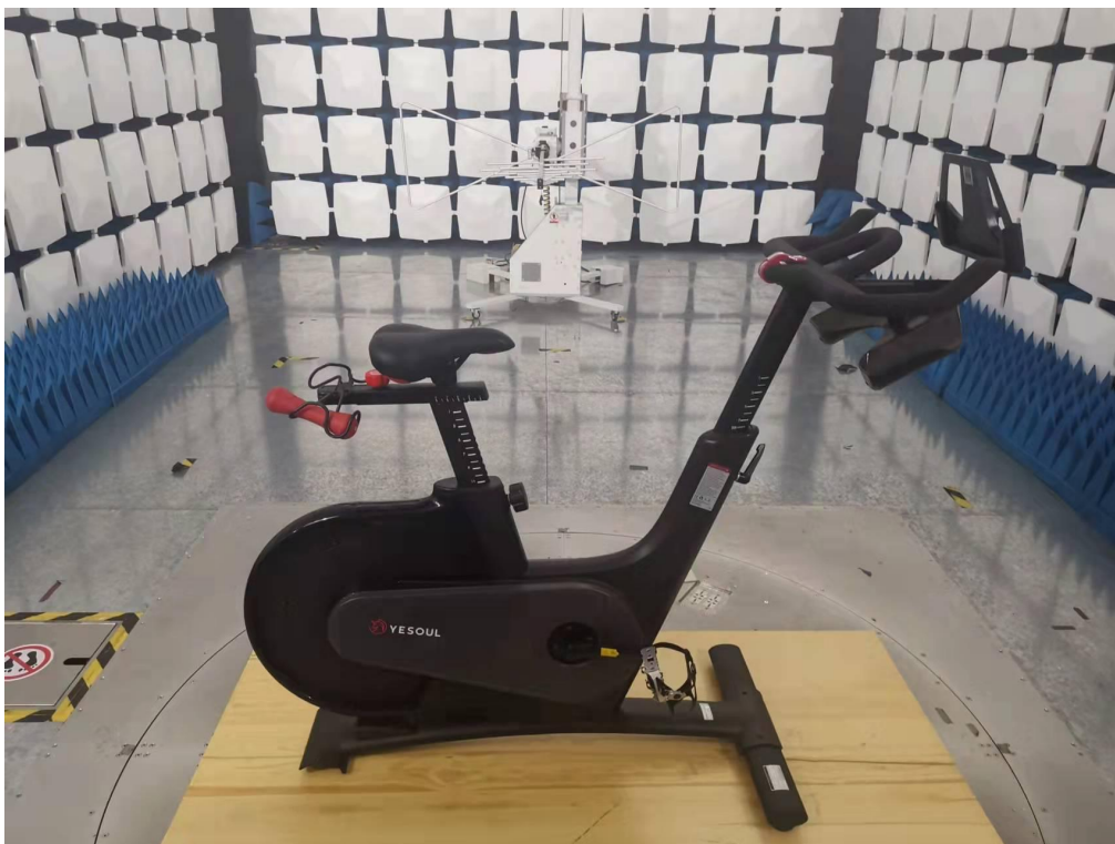
Below 1GHz for radiated emission test setup
