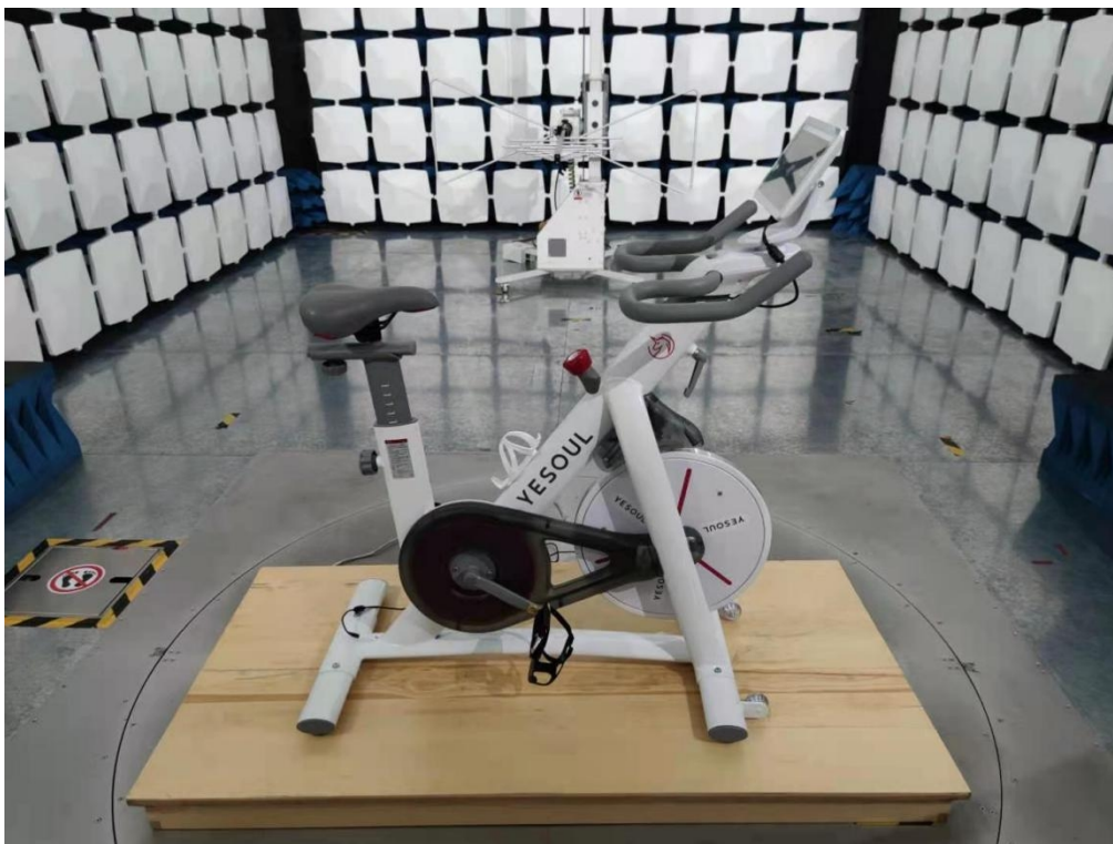
Below 1GHz for radiated emission test setup
