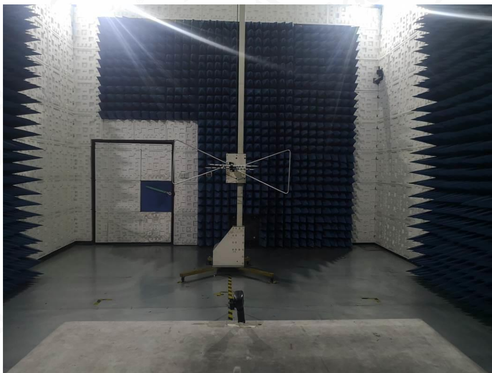
FCC RADIATED EMISSION TEST SETUP ABOVE 1GHZ
