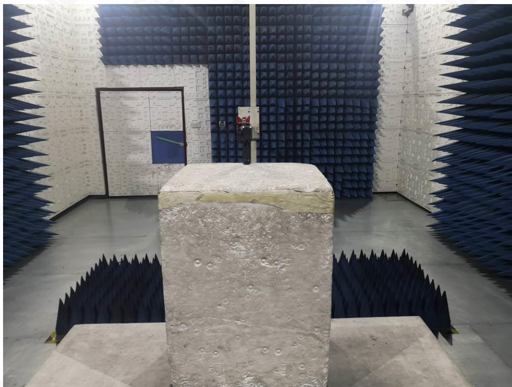
FCC RADIATED EMISSION TEST SETUP ABOVE 1GHZ
