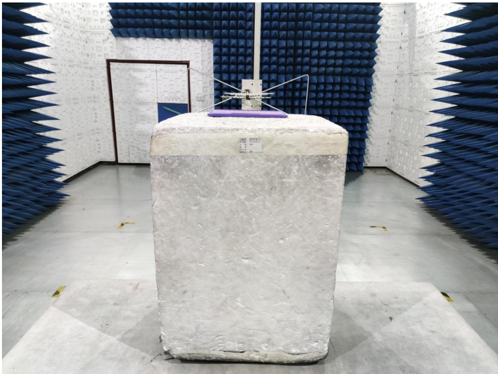
RADIATED EMISSION TEST SETUP ABOVE 1GHZ
