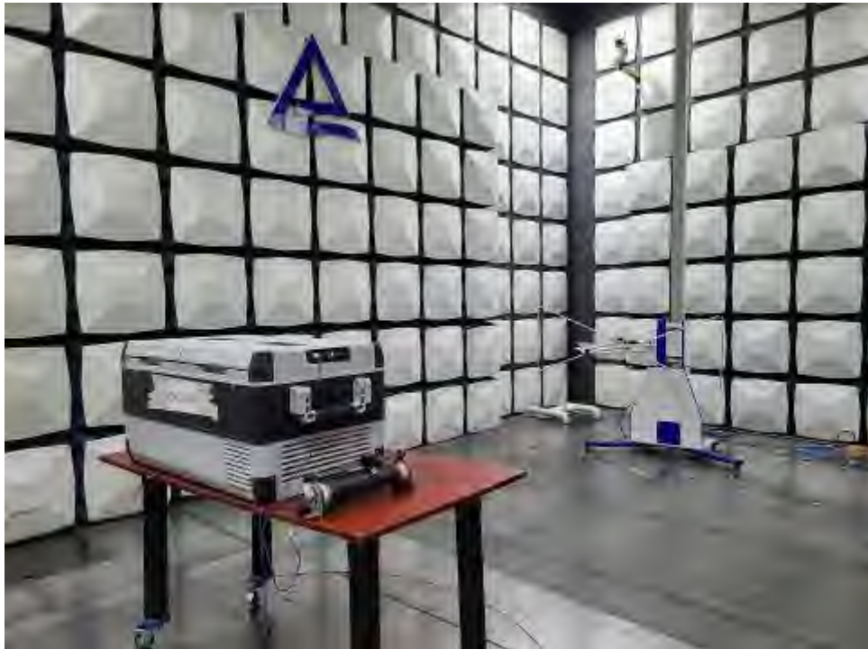
Photograph 2: Set-up for Radiated Spurious Emission, 1GHz - 18GHz
