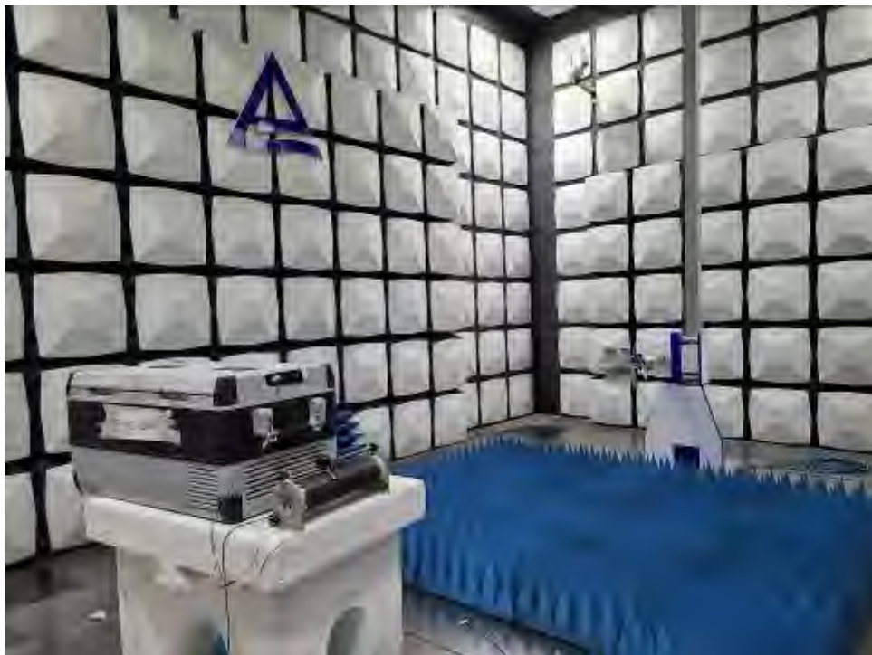
Photograph 2: Set-up for Radiated Spurious Emission, 1GHz - 18GHz
