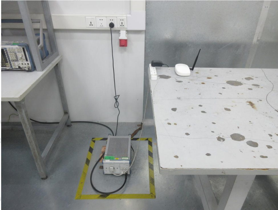
Photo of Power Line Conducted Emission Test
