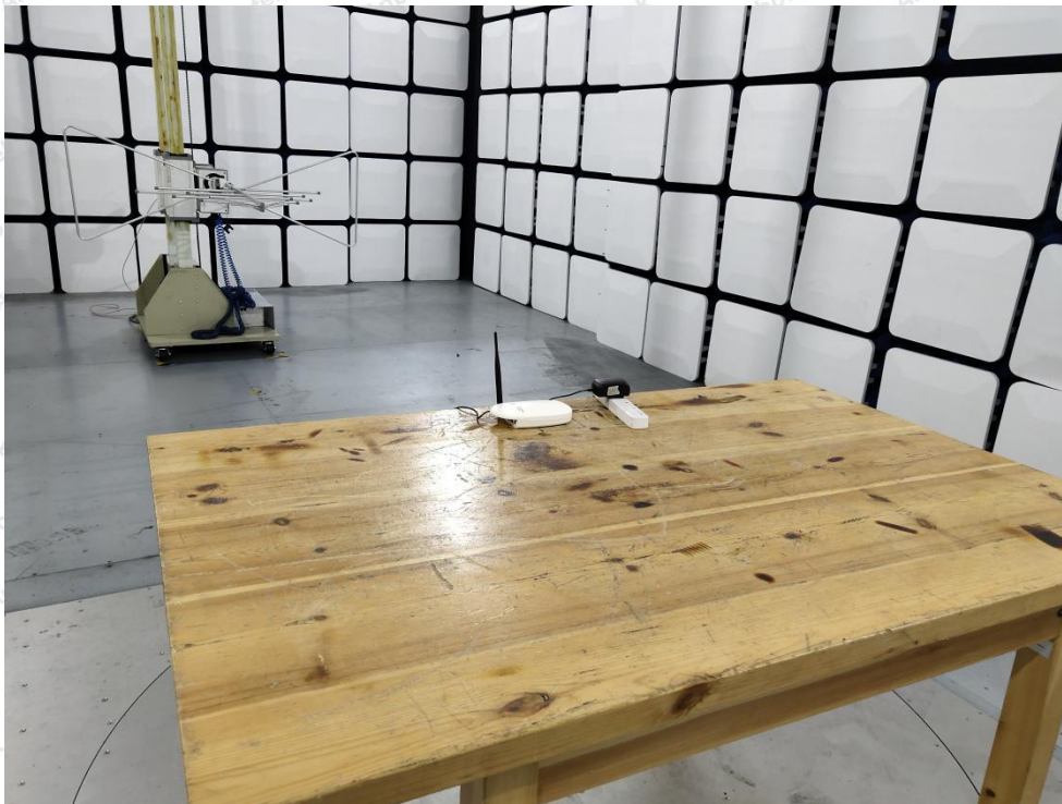
Photo of Radiation Emission Test
