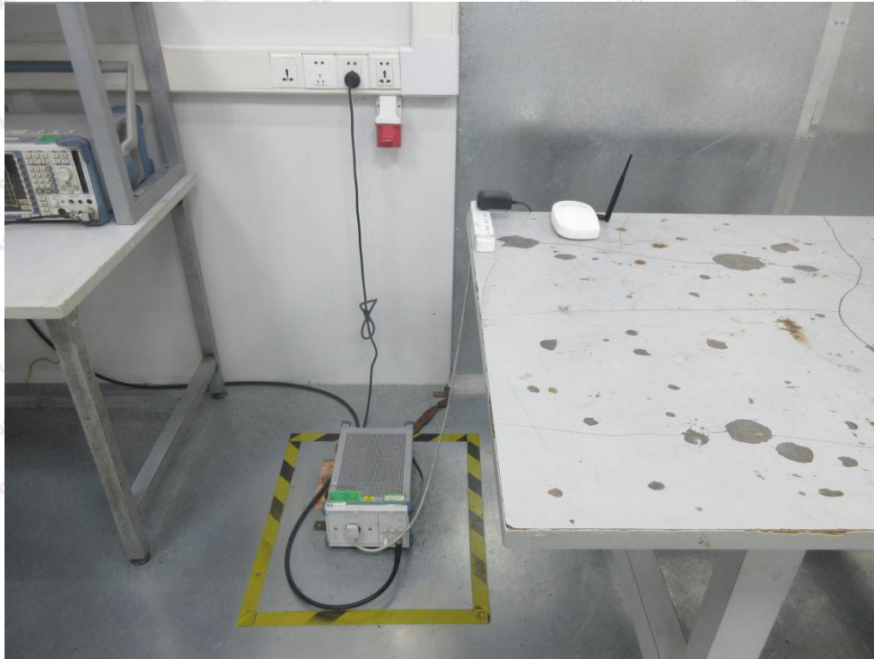
Photo of Power Line Conducted Emission Test
