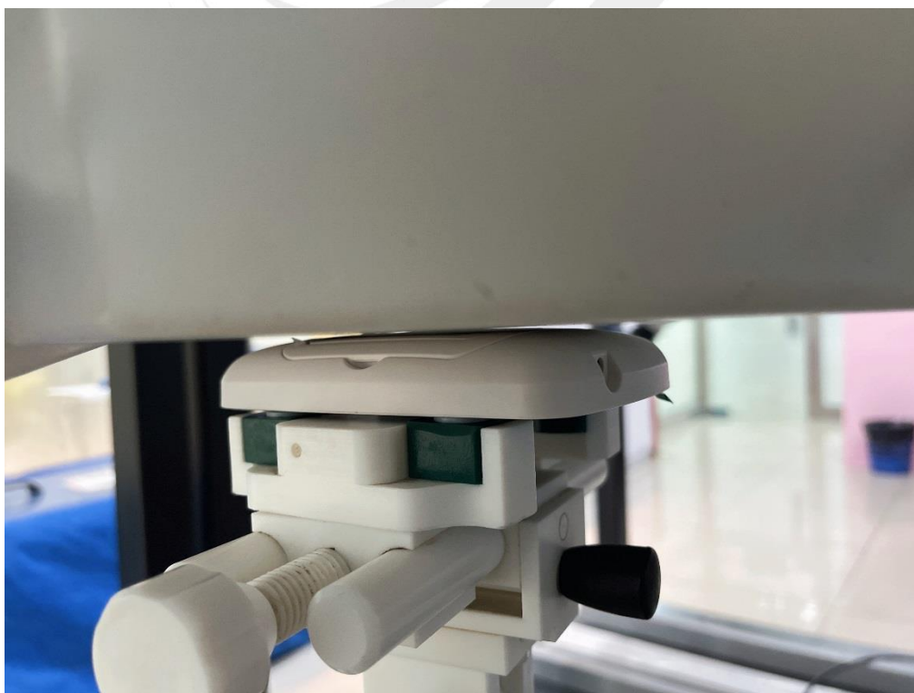
Body Back side(separation distance is 0mm)
