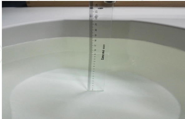
The Body Liquid of 2450MHz (15.3cm)
